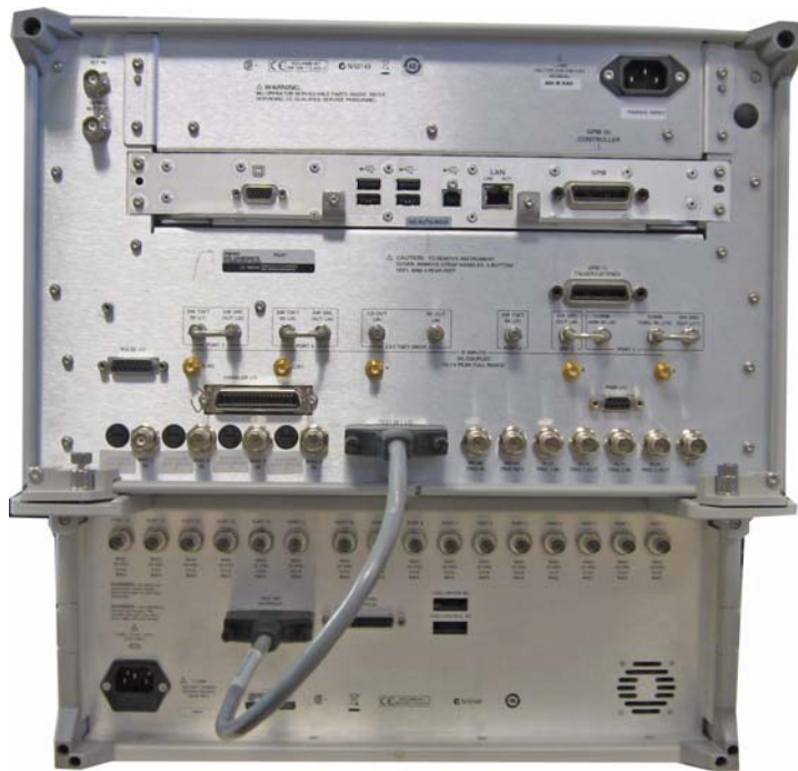
Figure 29 N5242A Test Set I/O Cable Connection
