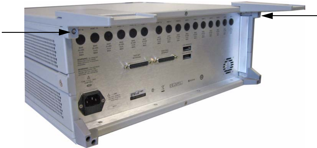
Figure 25 Install Locking Feet on U3042AE08
